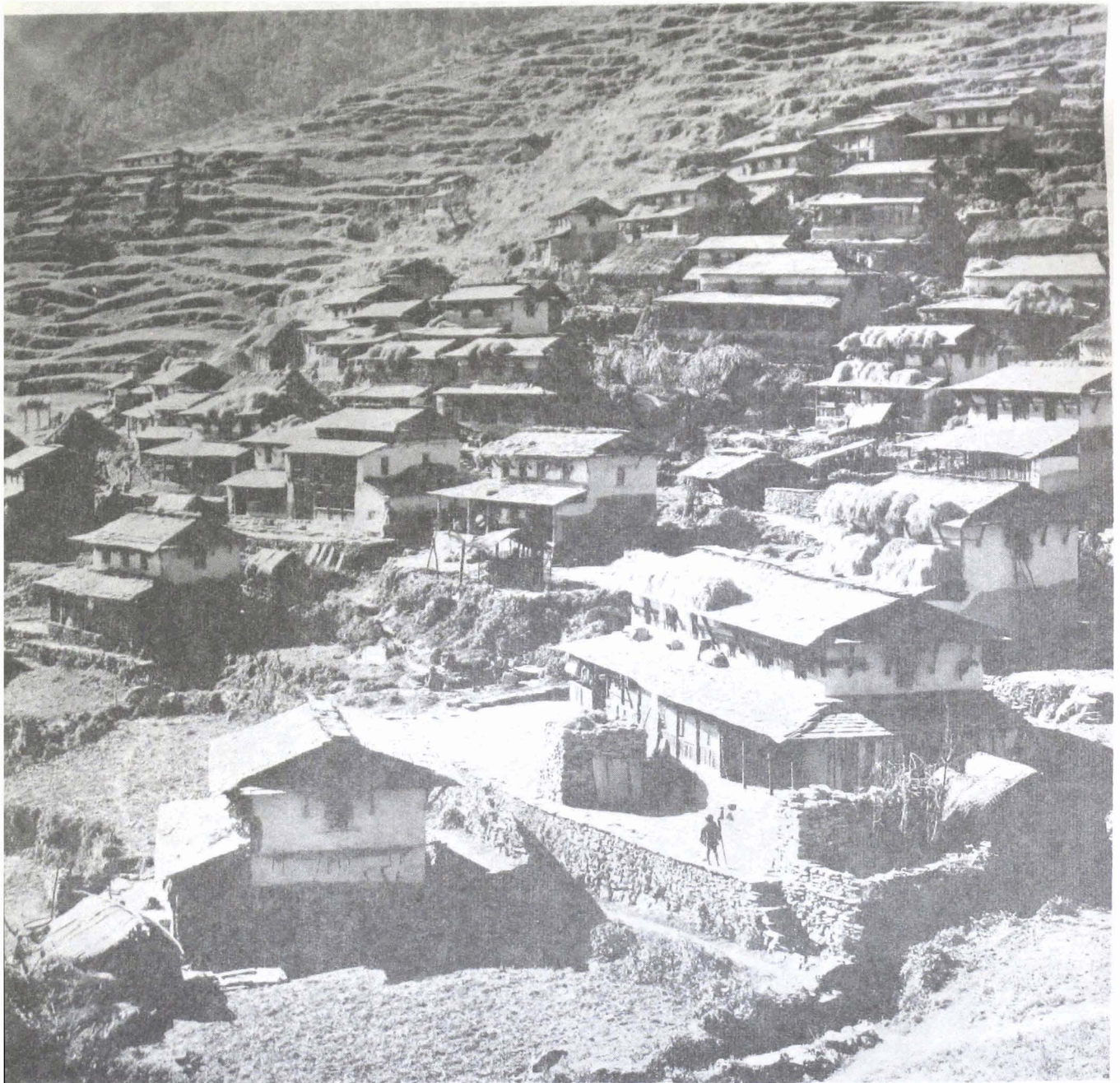
Fig. 4: Section of the settlement of Muri in the Mayangdi Khola, 2000 m above sea-level, photographed to the south. The houses are built with their longitudinal axis parallel to the contour lines on the slope. For the most part, they are roofed with flagstones and the outer walls are daubed. They have one- and two storey high loggias which, in some cases, surround the entire house. (18. 1. 1977, photo: M. Kuhle)
